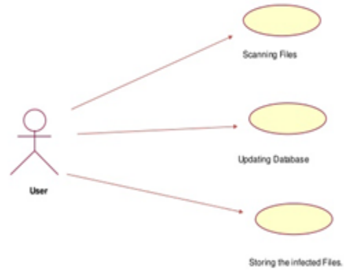
Fig. 2. Use Case Diagram: shows what all user can do. He can scan files for any malicious content, can update the signature database and can store the infected files in sandbox for isolation purpose.
